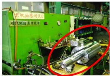
Fig.2. ATS hydraulic circuit modifications.
